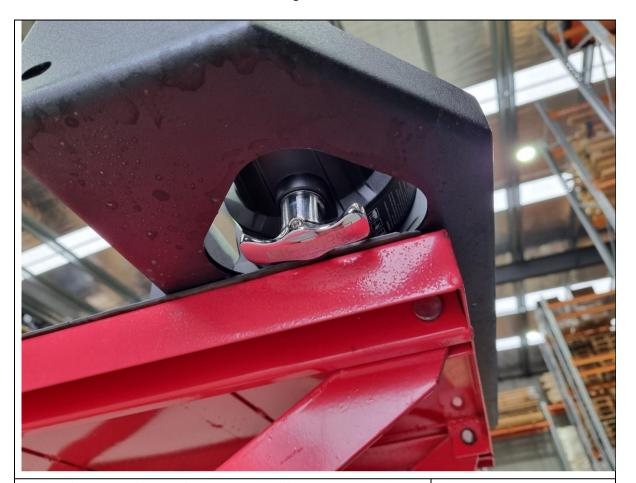
36. (OPTIONAL) When fitted with the Offroad Animal Pre Runner steel front bumper, the winch clutch lever can be accessed from below.
