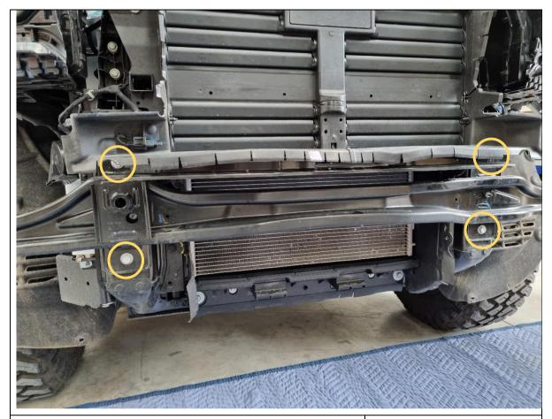
19. Using a 16mm socket or spanner, remove the 4x hex head bolts securing the impact beam to the body.
