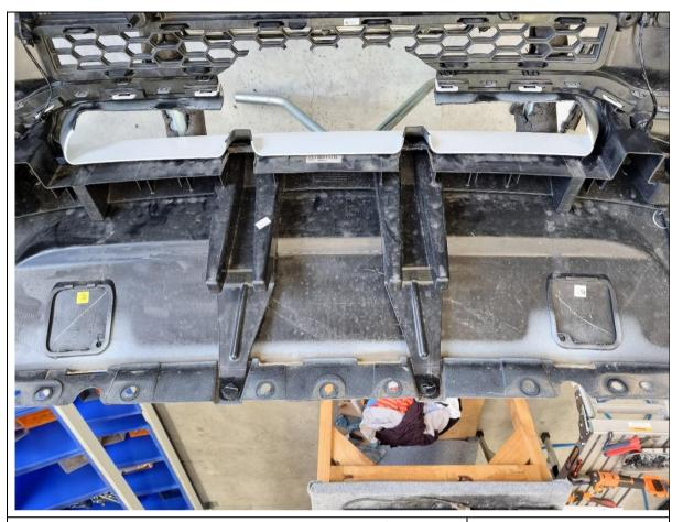
73. Reassamble the main bumper section, lower half and plastic inner support (Overland models only) back together using the original fasteners.
