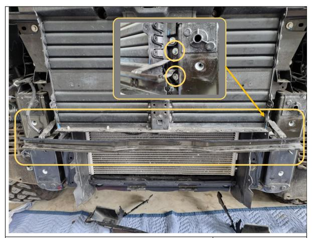
22. Remove the steel cross beam by removing the 4x 10mm hex head bolts securing it to the body (see inset).
