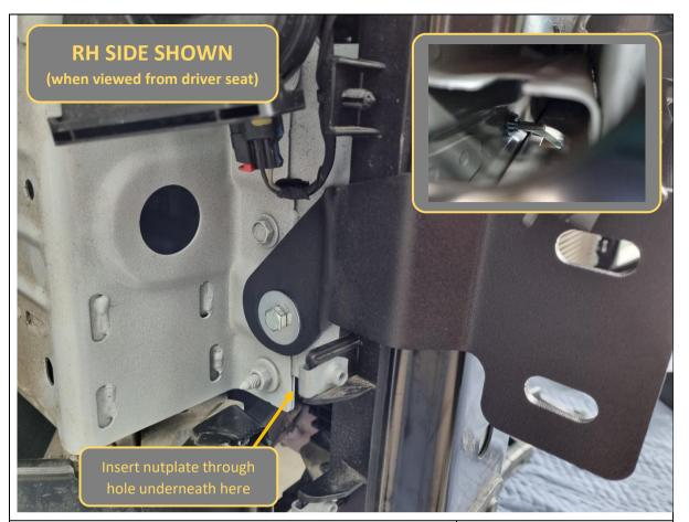
24. If no recovery points are to be fitted, loosely fit the chassis strap plate to the body by feeding 1x M8 lollipop nutplate through the rectangular hole (see inset) and secure with 1x M8x40 hex head bolt and large flat washer.
