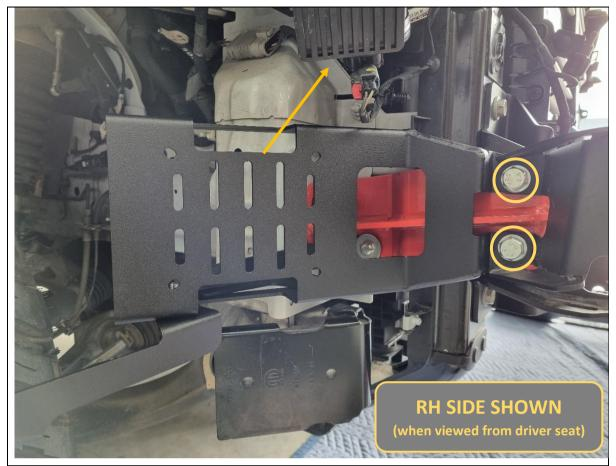
41. The winch control box relocation bracket can be fitted to either side of the vehicle.
