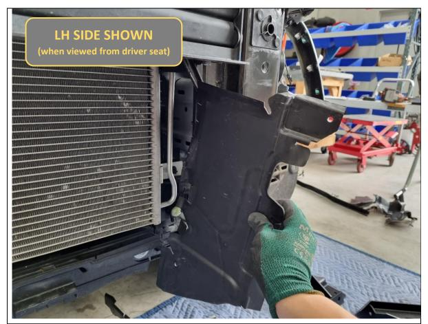
23. Unclip and remove the lower air dams with a flat head screwdriver or trim tool.
